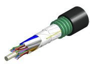
Fiber indoor/outdoor cable, LazrSPEED®, Mini Single Jacket/Single Armor, Riser/LSZH rated, 8 fiber, Gel-Filled, Stranded Loose Tube, Multimode OM3, Meters jacket marking, Black jacket color, B2ca flame rating
