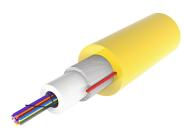
Fiber Indoor/Outdoor Cable, 24-fiber, singlemode G.652.D and G.657.Al, Gel-filled, yellow jacket color, Dca Flame Rating, Meters jacket marking, 2000 meters
