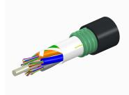
Fiber indoor/outdoor cable, LazrSPEED®, Single Jacket/Single Armor, Low Smoke Zero Halogen (LSZH), 48 fiber, Gel Filled , Stranded Loose Tube, Multimode OM3, Black jacket color, Meters jacket marking, Cca flame rating
