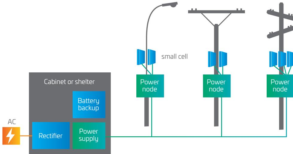
Figure 7. Example of a low voltage dc power solution
