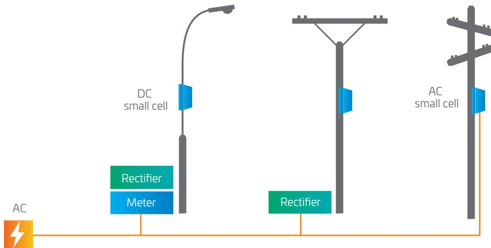
Figure 2. Example of utility grid power solution
