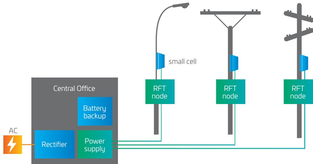
Figure 5. Basic configuration of an RFT circuit
