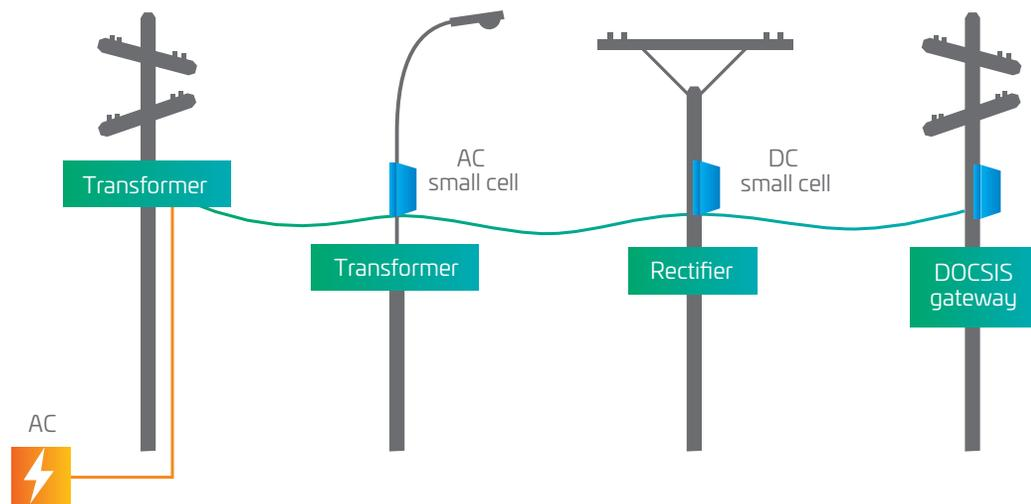
Figure 4. Example of an HFC power solution
