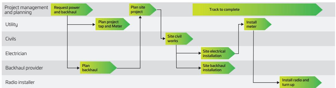
Figure 3. The typical process of connecting to the grid
