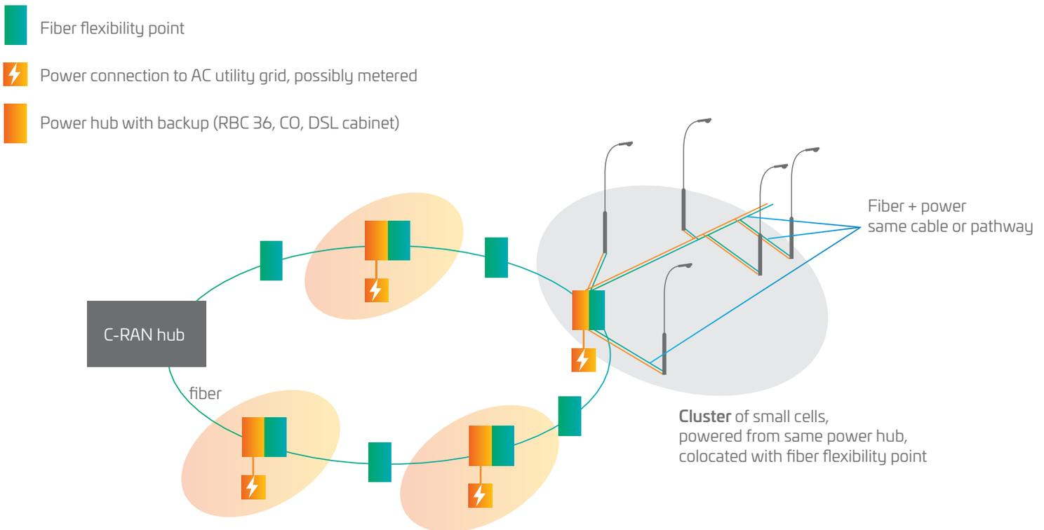
Figure 6. Cluster power solution in support of a C-RAN deployment
