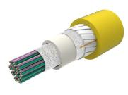
Fiber indoor cable, All-Dielectric, LSZH/Riser-Rated, Gel-Free, Central Tube Rollable Ribbon, 432 fiber, Singlemode G.657.A2/B2, Feet jacket marking, Yellow jacket color, Cca flame rating
