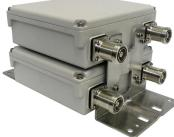
Twin Diplexer, LTE 800/GSM 900 AISG compatible, dc pass on Low port for unit 1 and High port for unit 2
