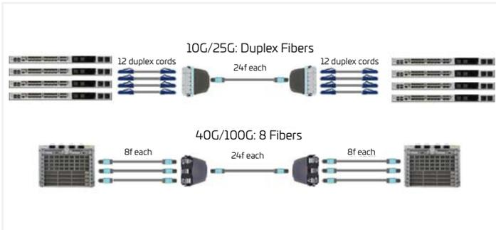
Figure 7: Cabling infrastructure supporting two-fiber applications to eight-fiber applications
