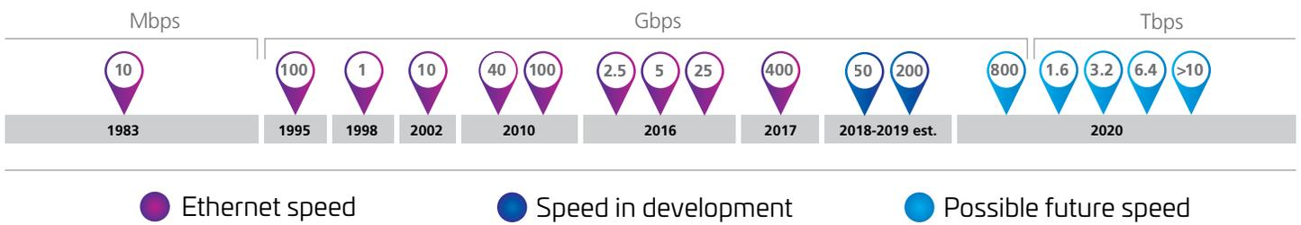
Figure 6: Roadmap for Ethernet speeds (source: Ethernet Alliance)
