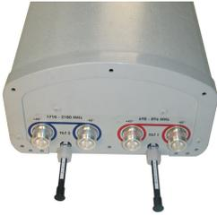
4-port sector antenna, 2x 698–896 and 2x 1710–2180 MHz, 65° HPBW, RET compatible
