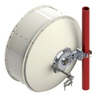
1.2 m | 4 ft Sentinel® High Performance Antenna, dual-polarized, 14.400– 15.350 GHz
