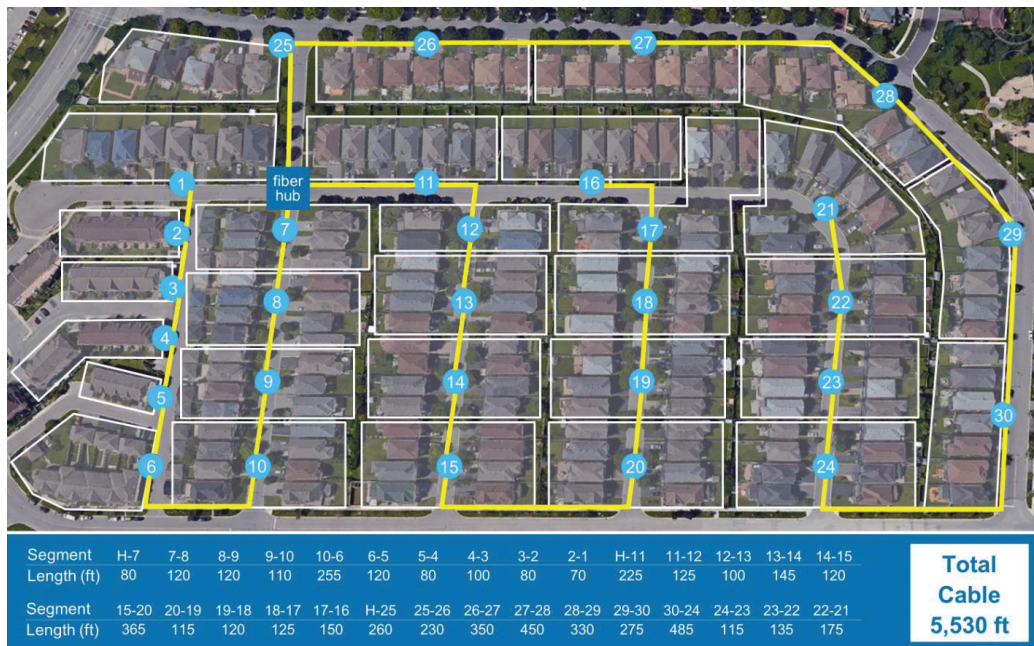
Figure 1B: Fiber Indexing uses a linear daisy-chain topology, with terminals that perform multiple functions
