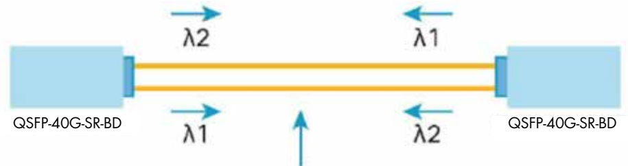
Duplex Multi-mode Fibre with LC Connectors at both ends
