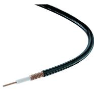
Heat Treated FSJ2RK-50, HELIAX® Superflexible Foam Coaxial Cable, corrugated copper, 3/8 in, black non-halogenated, fire retardant polyolefin jacket
