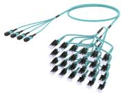
Ultra Low Loss ULL LazrSPEED® 550 MPO(Pinned) to LC/UPC Uniboot Ruggedized fanout Cable, 48-Fiber, LSZH, 12 fiber PmP 2.0 mm Dca
