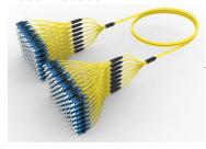
Ultra Low Loss ULL TeraSPEED® SC/UPC to SC/UPC Ruggedized fanout Cable, 96-Fiber, Plenum, 12 fiber PmP 2.0 mm Dca
