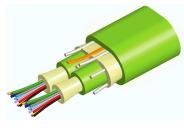
Fiber indoor cable, LazrSPEED®, Low Smoke Zero Halogen Riser MPO Trunk, 24 fibers, 12 fiber subunits, Multimode OM5, Gel-free, Feet jacket marking, Lime green jacket color, B2ca Flame rating
