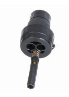
FOSC® Gel Sealing Kit for round splice closure port, sealing 2 cables with diameter between 7 and 11 mm
