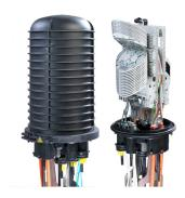
FIST® GCO2 Fiber Optic Splice Closure, Heat Shrink or Gold Gel Cable sealing, size BC, no pre-installed fiber trays, 6 round ports + 1 oval port, with test valve
