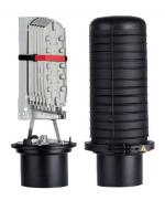
FOSC® 450 C6 Fiber Optic Splice Closure, Gel Cable sealing, pre-installed C ribbon tray, 6 cable attach., six ground feedthrough lugs, with test valve
