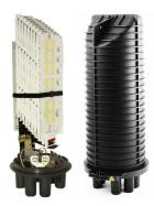
FOSC® 400 D5 Fiber Optic Splice Closure, Heat Shrink Cable sealing, two pre-installed 72-splice trays, cable blocking, ground feedthrough lugs, with test valve
