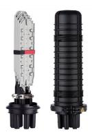
FOSC® 400 B4 Fiber Optic Splice Closure, Heat Shrink Cable sealing, one pre-installed 12-splice tray, ground feedthrough lugs, with test valve
