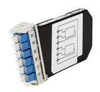
FMT MicroVAM Fiber Optic Monitoring Module, two 1x2 splitters, singlemode, FC/UPC, 90/10 split ratio
