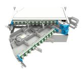
MFPS Fiber Optic panel, 2RU, 96 fibers/RU, splice/patch, ANT/front patch cords orientation to the right, 192 LC/APC, grade C
