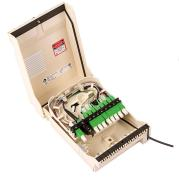
RapidFiber® Mini-RDT, 1x4 Indexing Terminal, 3.6mm Black Riser I/O cable, female MPO at far end, 300 ft
