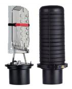
FOSC® 450 B6 Fiber Optic Splice Closure, Gel Cable sealing, one preinstalled 24-splice tray, 2 cable attachments, three ground feedthrough lugs, with test valve
