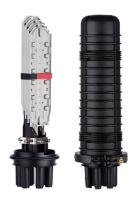
FOSC® 400 B4 Fiber Optic Splice Closure, Heat Shrink Cable sealing, two pre-installed 24-splice trays
