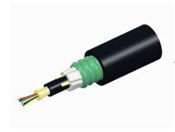
Fiber outdoor drop cable, Low Smoke Zero Halogen Single Jacket Single Armor Arid-Core, Singlemode G.657.A2/B2, Gel-free, Feet jacket marking, Black jacket color
