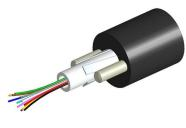
Fiber drop cable, TeraSPEED® Single Jacket All-Dielectric Arid Core, 12fiber, Singlemode G.652.D and G.657.A1, Gel-filled, Feet jacket marking, Black jacket color
