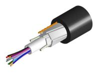
Fiber Indoor/Outdoor Drop Cable, LazrSPEED®, Low Smoke Zero Halogen Single Jacket, 8 fiber, All-Dielectric Arid-Core, Gel-filled, Multimode OM3, Feet jacket marking, Black jacket color, Dca flame rating
