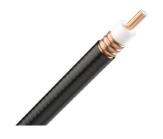
AVA5RK-50FX, HELIAX® Andrew Virtual Air™ Coaxial Cable, corrugated copper, 7/8 in, black, Non-halogenated, fire retardant polyolefin jacket B2ca-sl, d2,al (CPR testing is conducted annually please reference the website for latest classification)
