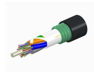
Fiber indoor/outdoor cable, LazrSPEED®, Single Jacket/Single Armor, Low Smoke Zero Halogen (LSZH), 24 fiber, Multimode OM4, Gel Filled, Stranded Loose Tube, Black jacket color, Meters jacket marking, Cca flame rating
