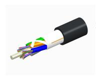
Fiber OSP cable, LazrSPEED® Single Jacket All-Dielectric, Gel-Free, Stranded Loose Tube, 24 fibers, Multimode OM5, Feet jacket marking, Black jacket color
