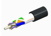
Fiber OSP cable, LazrSPEED® Single Jacket All-Dielectric, Gel-Free, Stranded Loose Tube, 24 fibers, Multimode OM5, Feet jacket marking, Black jacket color
