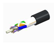
Fiber indoor/outdoor cable, TeraSPEED®/LazrSPEED®, Single Jacket All-Dielectric, LSZH, singlemode/multimode, 96 fiber, Gel-Free, Stranded Loose Tube, Feet jacket marking, Black jacket color, Eca flame rating
