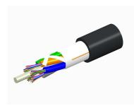
Fiber indoor/outdoor cable, LazrSPEED®, Single Jacket All-Dielectric, Low Smoke Zero Halogen (LSZH), Multimode OM4, 6 fiber, Gel-Free, Stranded Loose Tube, Feet jacket marking, Black jacket color, B2ca flame rating
