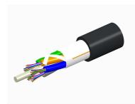
Fiber indoor/outdoor cable, LazrSPEED®, Single Jacket All-Dielectric, Low Smoke Zero Halogen (LSZH), Multimode OM5, 6 fiber, Gel-Free, Stranded Loose Tube, Feet jacket marking, Black jacket color, B2ca flame rating
