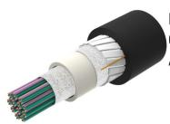
Fiber indoor/outdoor cable, All-Dielectric, LSZH Riser-Rated, Gel-Free, Central Tube Rollable Ribbon, 576 fiber, Singlemode G.652.D and G.657. Al, Feet jacket marking, Black jacket color, Cca flame rating
