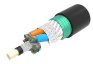
Fiber OSP cable, Outdoor Steel Armored, Gel-Free, Stranded Loose Tube Rollable Ribbon, 1440 fiber, Singlemode G.652.D and G.657.A1, Feet jacket marking, Black jacket color
