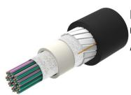
Fiber indoor/outdoor cable, All-Dielectric, LSZH Riser-Rated, Gel-Free, Central Tube Rollable Ribbon, 864 fiber, Singlemode G.652.D and G.657. Al, Feet jacket marking, Black jacket color, Cca flame rating
