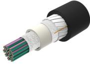
Fiber indoor/outdoor cable, All-Dielectric, LSZH Riser-Rated, 144 fiber, Gel-Free, Central Tube Rollable Ribbon, Singlemode G.652.D and G.657. A1, Feet jacket marking, Black jacket color, Cca flame rating
