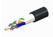
Fiber indoor/outdoor cable, LazrSPEED®, Single Jacket All-Dielectric, Low Smoke Zero Halogen (LSZH), 8 fiber, Gel-Free, Stranded Loose Tube, Multimode OM3, Black jacket color, Feet cable marking, Eca flame rating
