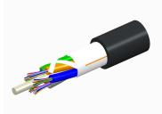
Fiber OSP cable, LazrSPEED® Single Jacket All-Dielectric, Gel-Free, 4 fiber, Stranded Loose Tube, Multimode OM4, Feet jacket marking, Black jacket color
