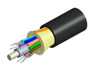
Fiber Indoor/Outdoor cable, LazrSPEED®, Low Smoke Zero Halogen Riser Distribution Cable, 4 fiber single-unit, Gel-free, Multimode OM4, Feet jacket marking, Black jacket color, Dca flame rating
