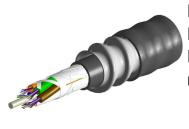
Fiber indoor/outdoor cable, TeraSPEED® Inner LSZH, Mini Stranded Loose Tube, 144 fiber, Riser Rated, Gel-filled Subunits with Aluminum Interlocking Armor, Singlemode G.652.D and G.657.A1, Feet jacket marking, Black jacket color
