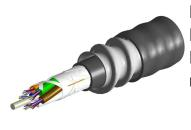
Fiber indoor/outdoor cable, TeraSPEED® Inner LSZH, Mini Stranded Loose Tube, 96 fiber, Riser Rated, Gel-Filled Subunits with Aluminum Interlocking Armor, Singlemode G.652.D and G.657.A1, Feet jacket marking, Black jacket color
