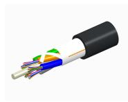
Fiber OSP cable, TeraSPEED® Single Jacket All-Dielectric, Gel-Free, Stranded Loose Tube, 72 fibers, Composite OM1 and G.652.D and G.657. Al, Feet jacket marking, Black jacket color
