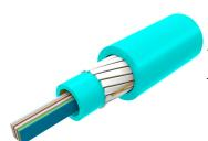
Fiber Indoor Cable, Multimode OM3 bend insensitive, 36 fibers, Plenum, All-Dielectric Central Tube Ribbon, Gel-free, Feet jacket marking, Aqua jacket color
