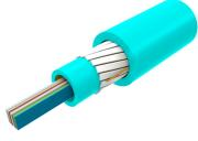
Fiber Indoor Cable, Multimode OM3 bend insensitive, 24 fibers, Plenum, All-Dielectric Central Tube Ribbon, Gel-free, Feet jacket marking, Aqua jacket color
