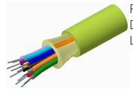
Fiber indoor cable, LazrSPEED® Low Smoke Zero Halogen Riser Distribution, 12 fiber single-unit, Multimode OM5, Feet jacket marking, Lime green jacket color, Dca flame rating
