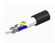
Fiber OSP cable, TeraSPEED® Single Jacket All-Dielectric, 144 fiber, Gel-Free, Stranded Loose Tube, Composite OM3 and G.652.D and G.657.Al, Feet jacket marking, Black jacket color
