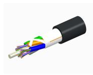
Fiber OSP cable, TeraSPEED® Single Jacket All-Dielectric, Gel-Free, Stranded Loose Tube, 18 fibers, Composite OM3 and G.652.D and G.657. Al, Feet jacket marking, Black jacket color
